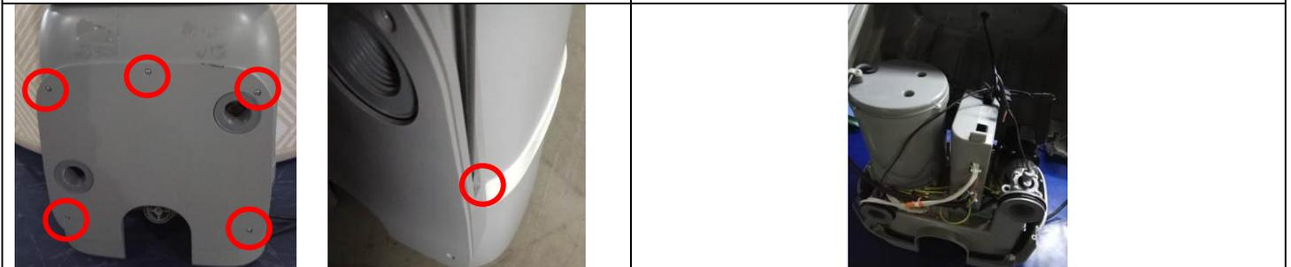
3、 Loosen five screws (ST4\*15) from the rear cover of the cabinet; Loosen two screws (ST4\*15) from the base of the cabinet
